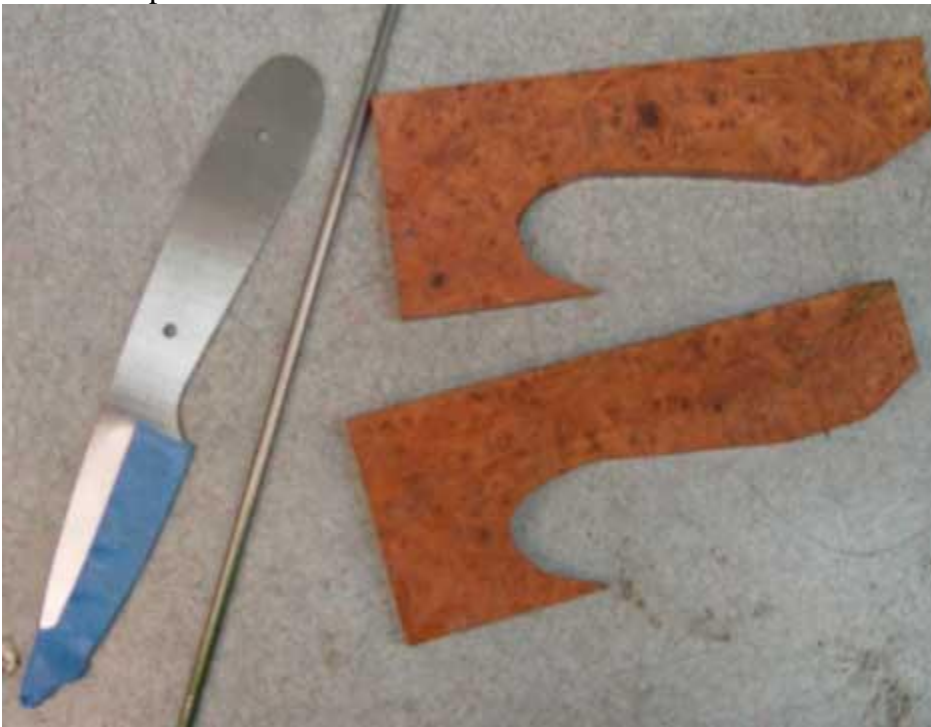
The scales must be sanded flat. A cheap and easy way to do this is a piece of glass and 220X paper
