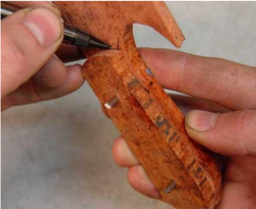
Scribing the first scale's top profile onto the second scale
