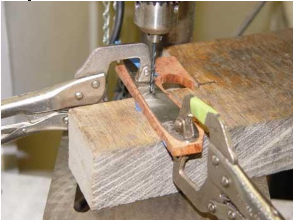
Drilling the scale with a 1/8" bit
