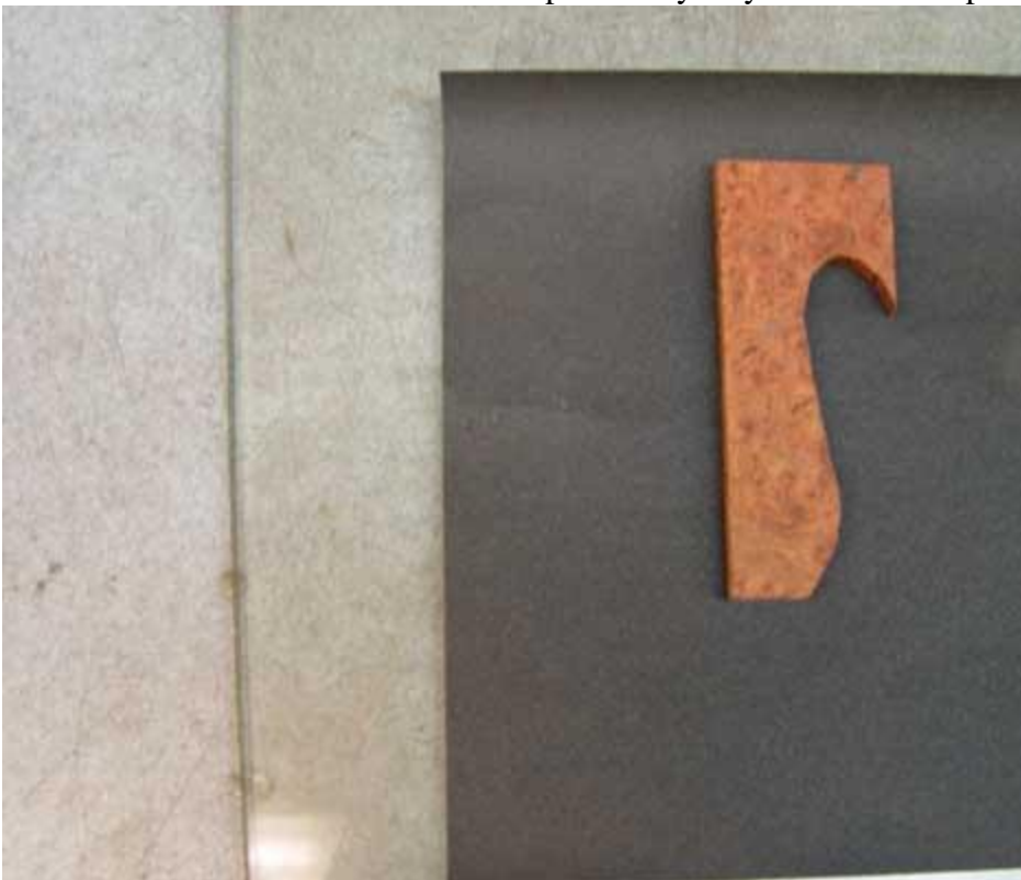
The scales must be sanded flat. A cheap and easy way to do this is a piece of glass and 220X paper
