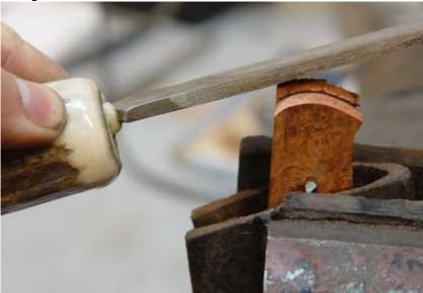
Filing the second scale to match the first
