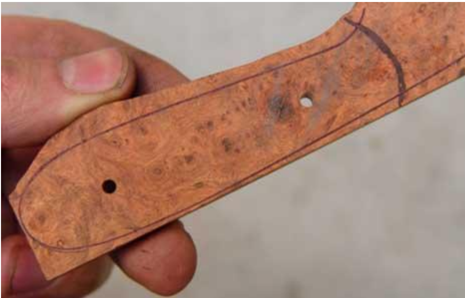
Tang outline drawn onto scale, including the top arch
