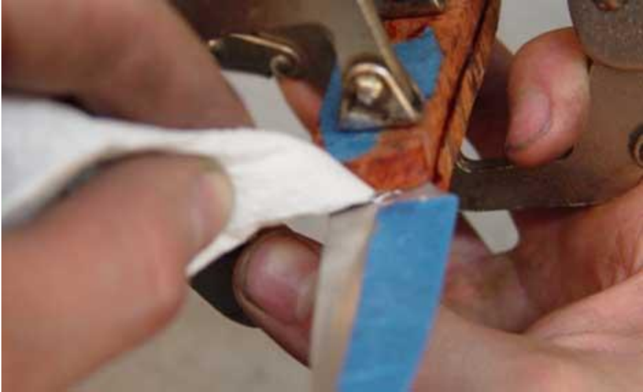
Cleaning the epoxy from the front of scales and blade with angled stick and paper towel
