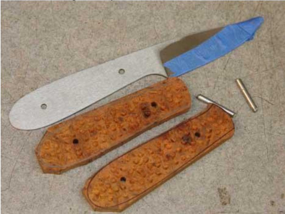
Blade, scales, and pins, ready to roll
