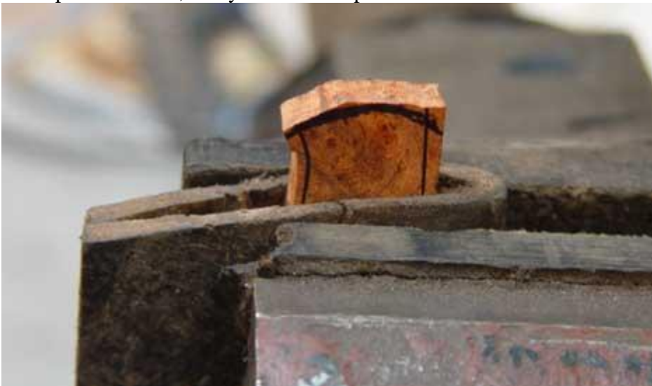
Scale placed in vise, ready to file the top down to line
