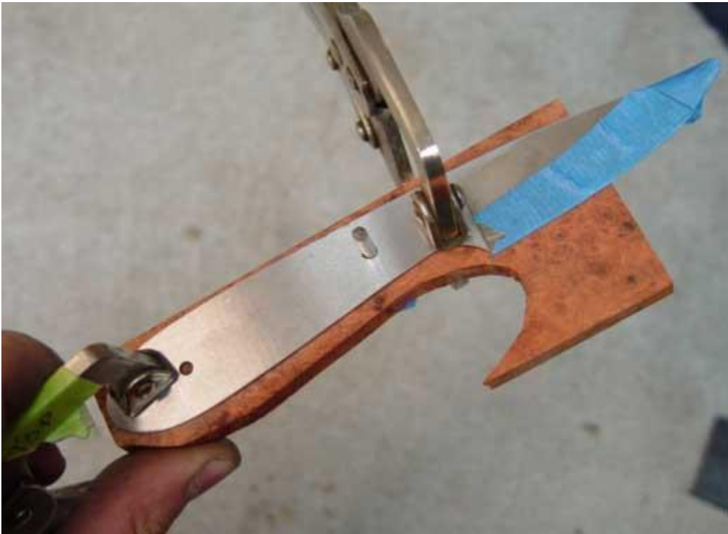
One hole is drilled, and then a pin is placed through that hole before moving on
