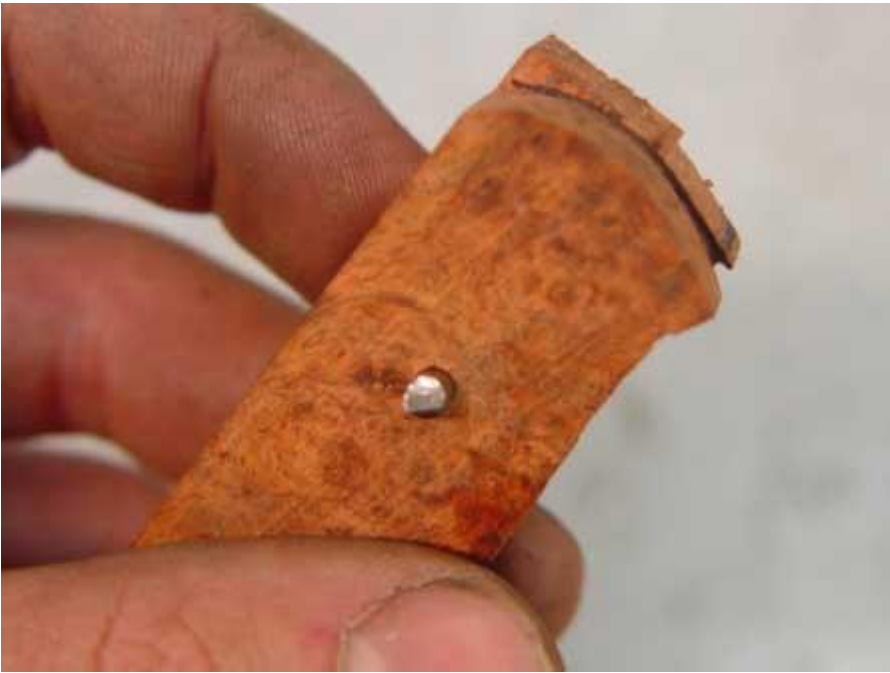
Pin the scales together
