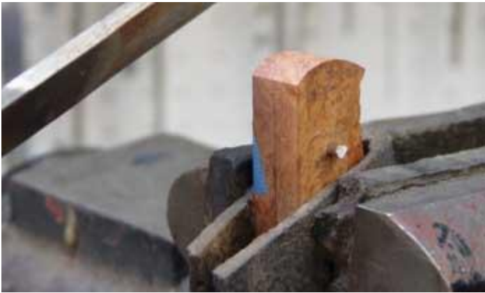
Scales filed down to the same profile
